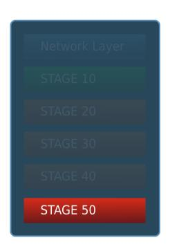
This stage triggers the associated callbacks every time a TCP connection is closed by a protocol, scheduler timeout or due to any network anomaly found.
