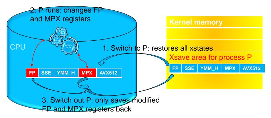
Example of how only modified FP and MPX registers are detected and saved
