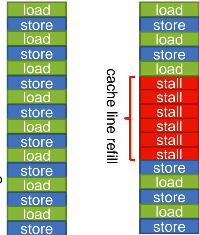
In reality can happen for both load and store, due to **allocate on write** cache line allocation policy
